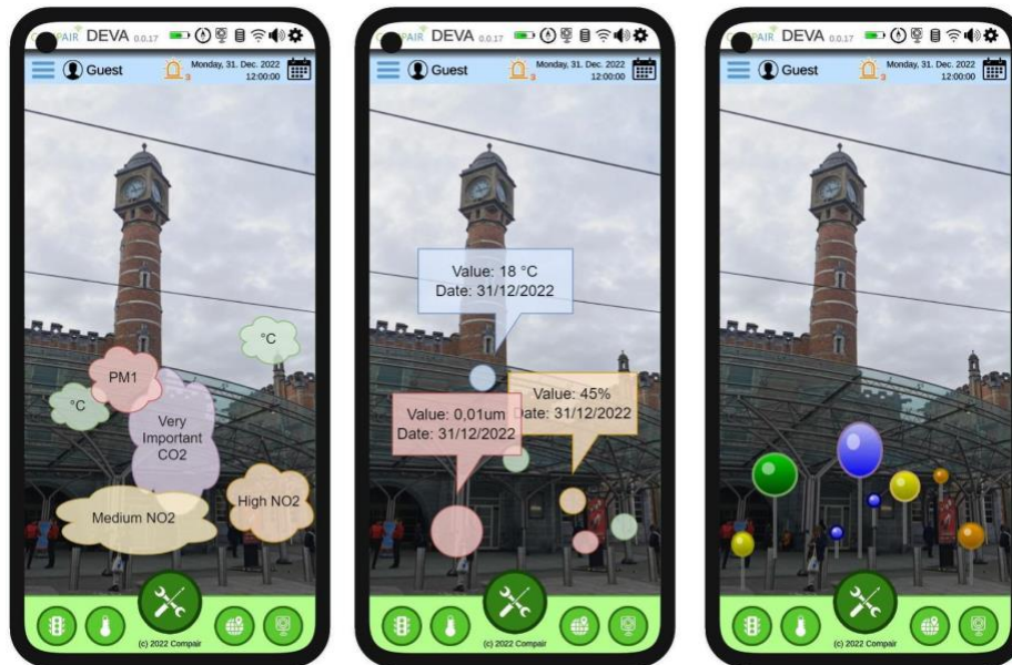
Figure 23: Examples of different visualisations of sensor data: (f.l.t.r.) clouds or point clouds, text or values, 3D pins
