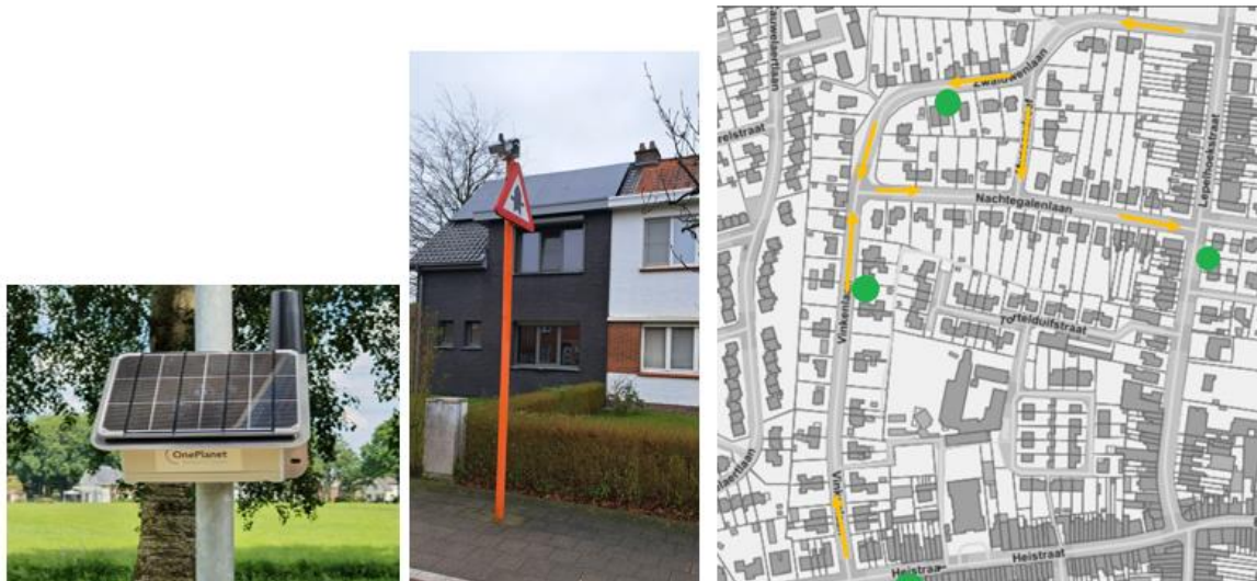
Figure 44: NO 2 -sensor box (left), NO 2 -sensor box in Sint-Niklaas (middle), locations of the sensor boxes in Sint-Niklaas (right)
