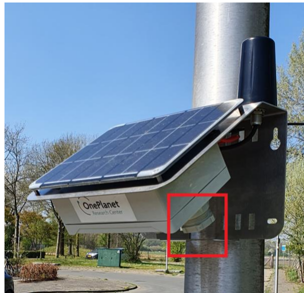
Figure 2.3 Location of electrochemical NO 2 sensor (Alphasense A43F) on the OnePlanet NitroSense device (Source: OnePlanet Research Center).
